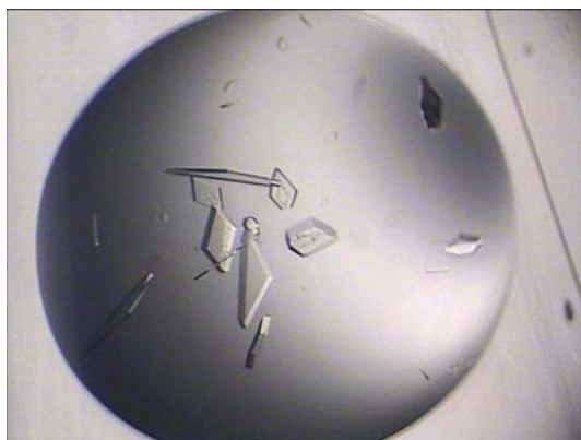
Figure 5 Sitting drop (2 \mu l) image collected by the imaging system at PAL resolution (768 \times 576 pixels).
